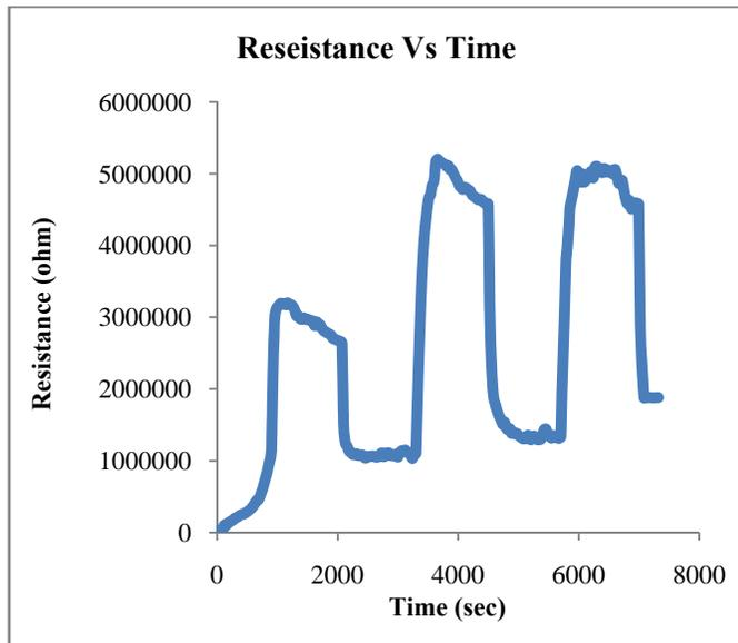
Fig. 8: Resistance response of PANI doped with HCl to 100 ppm ammonia gas.
