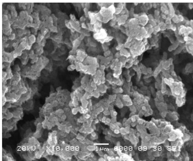
Fig. 4: SEM image of PANI doped with HCl (mag.10000)
