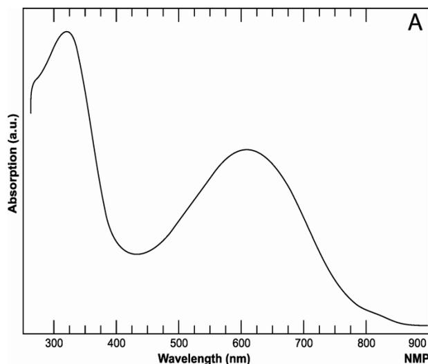
**Fig. 6: UV Spectra of PANI doped with HCl**
