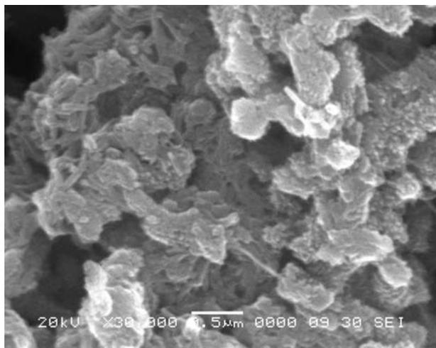
**Fig. 5: SEM image of PANI doped with HCl (mag.30000)**
